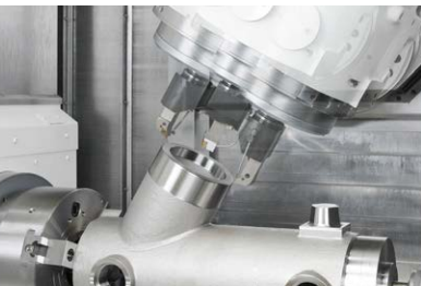
Turning can be done from a inclined axis
