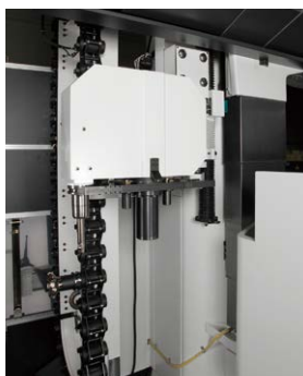
Next tool readied during machining operation
