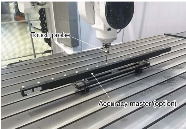
Automatic measurement of ball beam by touch probe
