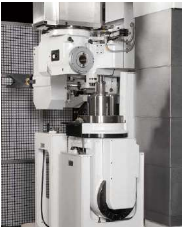
Changings heads: B-/C-axis universal index to 90° angular
