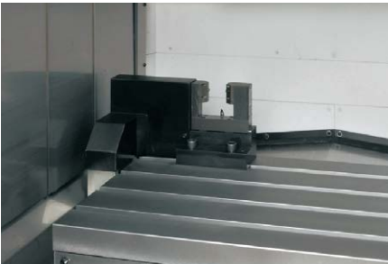
Auto tool length compensation (laser sensor) Measurements on minimum 0.1-mm drills possible during rotation
